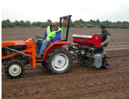
Figure 4. The Grassy Groundcover Restoration Project seeder in action. Seed is sown onto cultivated bed (developed by the seeder) then lightly covered and pressed into the soil.
