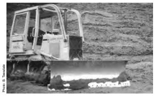
Bulldozers have been used to deep scalp the slopes for hand sowing.
