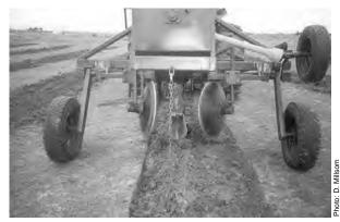
The Saltbush Seeder creates the m-profile for sowing in heavy soils in semi-arid areas and saline depressions
