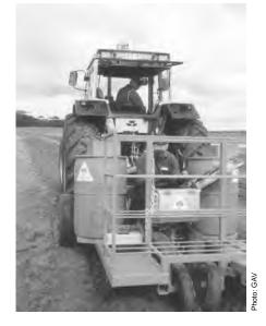
The Waikerie Tree Planter is a mechanical planter used for cell tray seedlings in specific soil types.
