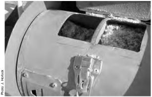
If the direct seeding machine you are using has two or three seed boxes, which allow different depths of sowing, sow large seeds at no more than 15 millimetres deep and sow small seeds on the surface. The use of the press wheel on machines will ensure good seed to soil contact.
