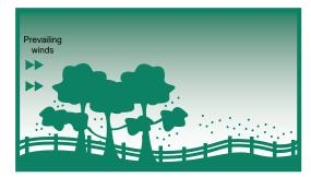
Extend the fence line out to the lee side of the trees so that the seeds fall inside the fenced area but beyond the tree canopy or 'drip-line'.
