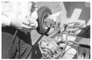
Hydraulics operated from cabin using battery powered motor
