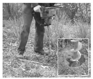
Mechanical auger used to create holes for planting
