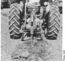
Deep ripping using a single type ripper to achieve loosened and friable soil conditions
