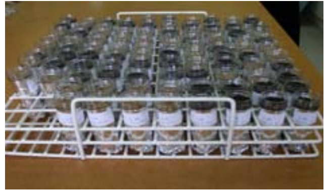
Plate 3 Foil covered tubes labelled and ready for the incubation cabinet. Photo Glenys Rose August 2009
