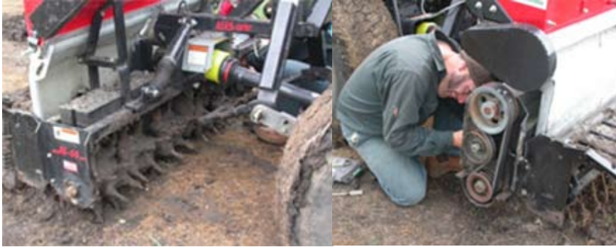
Sticky mud causes problems on our seeder-tines. Nothing Mr R White can't attend to by drawing on earlier life-skills
