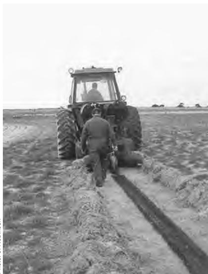
The Rodden III Scalping Seeder applying bitumen mulch in the Wimmera
