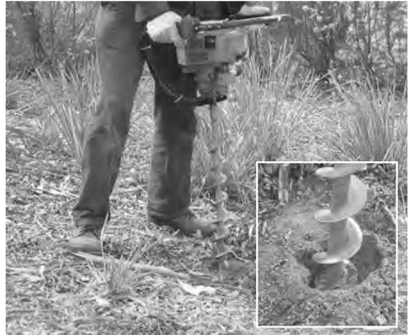
Mechanical auger used to create holes for planting
