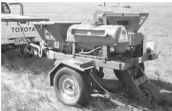
A variety of direct seeding machinery is available. They all use, essentially, the same process: scalping 25 to 50 millimetres of topsoil to form a weed free strip, cultivate the scalp line to create a seedbed, deposit seed in or on the seedbed and, except in sticky wet soils, use a press wheel to ensure good seed to damp soil contact.
