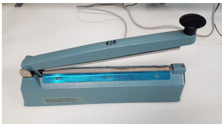
Figure 7. Benchtop (left) and foot operated (right) heat sealer for sealing plastic or foil bags. (Photos: L. Commander)
