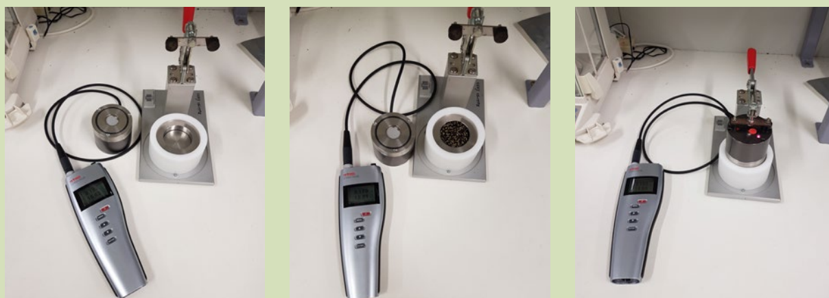
Figure 6. A hygrometer (left to right) without seed; once seed has been placed inside the sample chamber; closed to take the measurement. (Photos: L. Commander)
