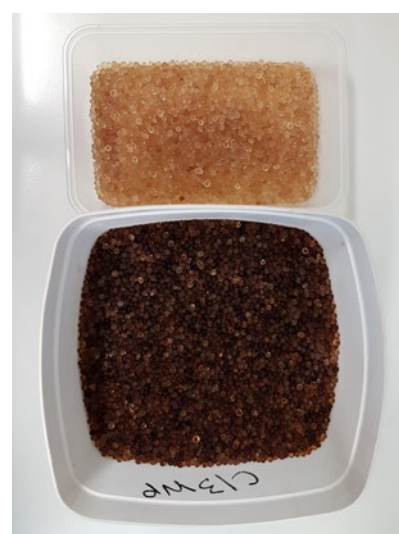
Figure 4. Silica gel with indicating dye. For these beads, a light orange colour indicates active beads and a dark colour indicates saturated beads that require re-drying. (Photo: L. Commander)
