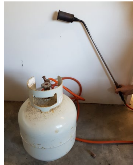
Figure 12. An LPG heating torch may be useful to open dehiscent fruits such as Banksia . (Photo: L. Commander)
