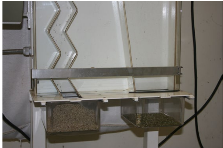
Figure 15. A zig-zag aspirator or vacuum separator can separate material based on weight. The seed lot is placed in the funnel at the top, and is fed into the main part of the machine via a vibrating channel. The lighter material (in this case the chaff) falls down the column shaped like a 'zig zag' and into the removeable Perspex tray on the left, whereas the heavier material (the seeds), are sucked over the top of the channel and fall down into the tray on the right. (Photos: L. Commander)
