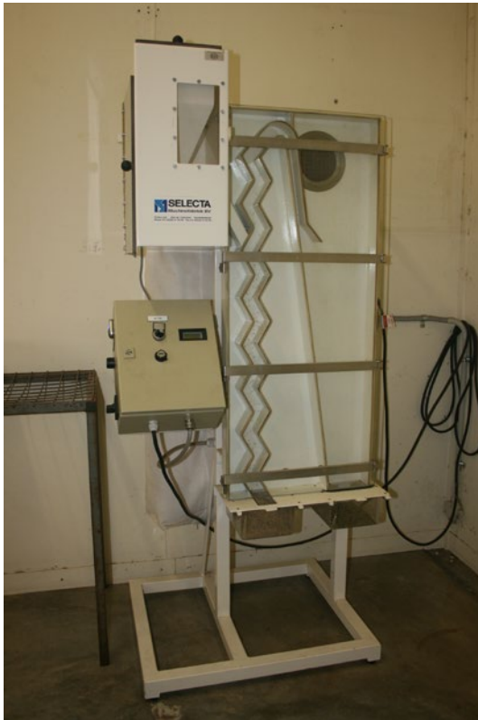
Figure 15. A zig-zag aspirator or vacuum separator can separate material based on weight. The seed lot is placed in the funnel at the top, and is fed into the main part of the machine via a vibrating channel. The lighter material (in this case the chaff) falls down the column shaped like a 'zig zag' and into the removeable Perspex tray on the left, whereas the heavier material (the seeds), are sucked over the top of the channel and fall down into the tray on the right. (Photos: L. Commander)
