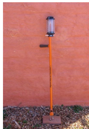
Figure 12. A hand seeder. (Photo: D. Carr)
