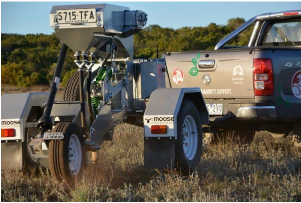
Figure 6. Moose seeder, which is an update of the Burford seeder. (Photo: T. Zwierson)
