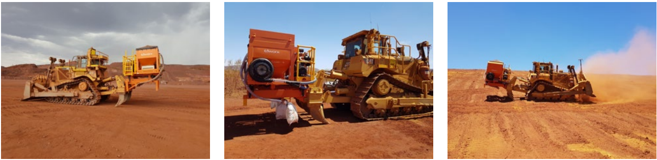
Figure 14. Air seeder attached to the back of a D9 for use on rocky soils and slopes up to 20 degrees, capable of metering a large range of native seeds. (Photos: N. Ellwood)
