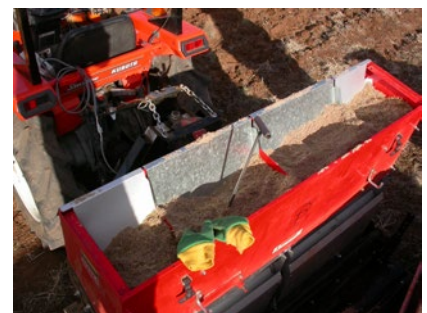
Figure 8. Grassland seeder developed by Paul Gibson-Roy for the Grassy Groundcover Restoration Project. It utilises a First Products Aerovator from the USA. The seed box is modified to deliver as many species as wanted. It does not use drill lines but drops seed as a curtain. (Photo: P. Gibson-Roy)
