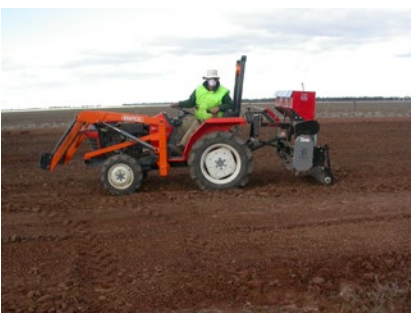
Figure 8. Grassland seeder developed by Paul Gibson-Roy for the Grassy Groundcover Restoration Project. It utilises a First Products Aerovator from the USA. The seed box is modified to deliver as many species as wanted. It does not use drill lines but drops seed as a curtain. (Photo: P. Gibson-Roy)
