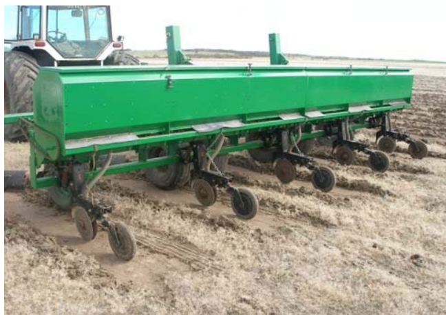
Figure 9. Row seeder. (Photo: P. Gibson-Roy)
