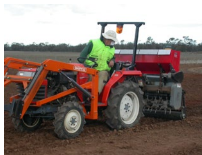
Figure 8. Grassland seeder developed by Paul Gibson-Roy for the Grassy Groundcover Restoration Project. It utilises a First Products Aerovator from the USA. The seed box is modified to deliver as many species as wanted. It does not use drill lines but drops seed as a curtain. (Photo: P. Gibson-Roy)
