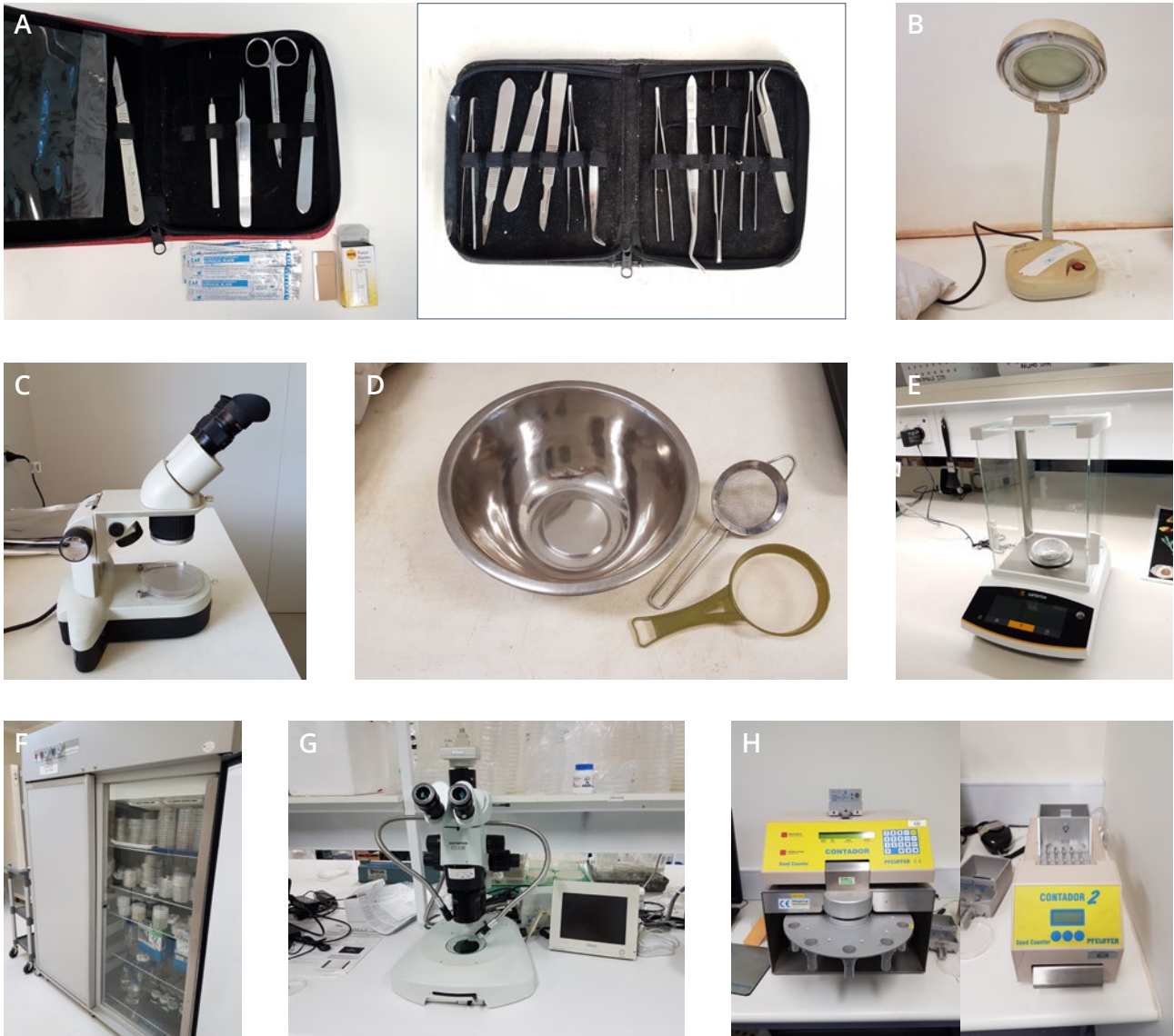
Figure 19. (A) Dissecting equipment including scalpels, forceps and razor blades. (B) Bench magnifier with a light. (C) Dissecting microscope. (D) Sieves and containers for separating seed from chaff for purity testing. (E) A balance used for weighing seeds. (F) Temperature and light controlled cabinet for incubating seeds for germination testing. (G) Microscope with a camera attached for taking photos of seeds. (H) Mechanised seed counters. (Photos: L. Commander)
