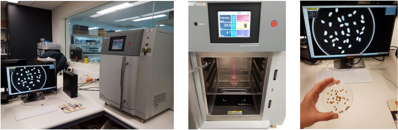
Figure 11. An X-ray cabinet used for seed fill testing with an attached computer showing the image. The shelf in the cabinet can be adjusted up or down according to the number and size of the seeds. (Photos: L. Commander)
