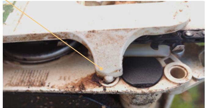
Throttle trigger Throttle lockout
